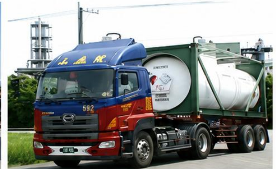
ISO Tank Container Truck
